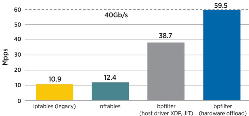
What becomes obvious is the remarkable performance improvement between bpfILTER, iptables and nftables; a 3.5X improvement over iptables and a 3.1X improvement over nftables (~6X and ~5X respectively with hardware offload). More importantly, the test with transparent hardware offload provided line rate performance with zero impact to the host CPU, as the SmartNIC performed the processing needed to drop packets.
