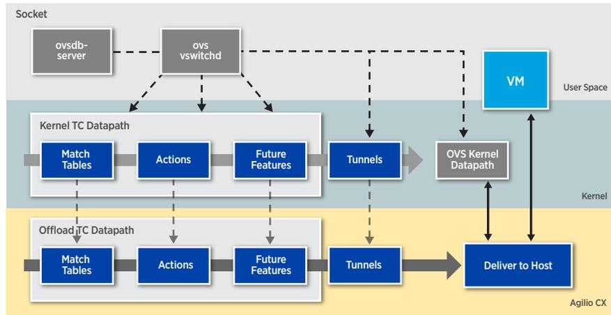
Figure 5: The Agilio transparent OVS-TC offload architecture
