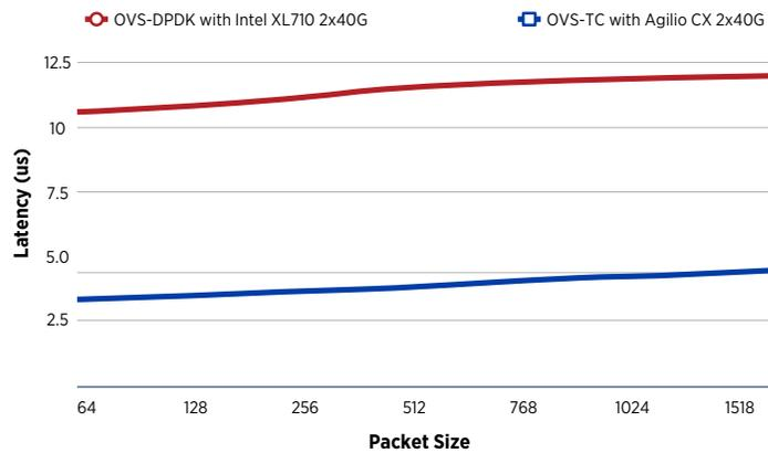
Figure 10: 2.5X lower latency with Agilio CX
