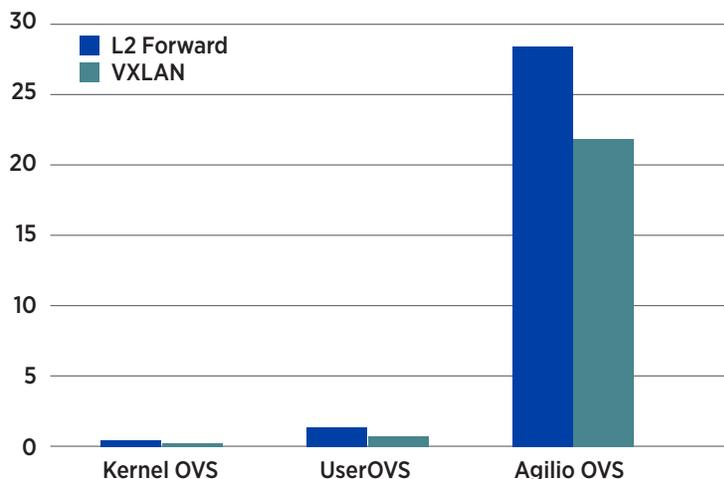
Figure 7. Normalized Performance (MPPS per single x86 Core)
