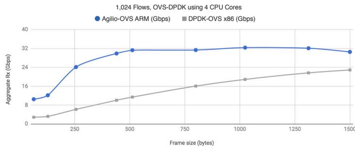
A comparison was performed between a solution combining Qualcomm's Centriq 2400 Processor in a server with an Agilio CX SmartNIC and Agilio OVS 2.6 software, against a solution combining Intel's E5-2630 Processor in a server with an Intel XL-710 NIC and DPDK OVS 2.6 software. VNFs were configured to run on each server and perform packet forwarding based on MAC address. Maximum VXLAN tunneled traffic throughput into and out of the server was measured as a function of packet size.
